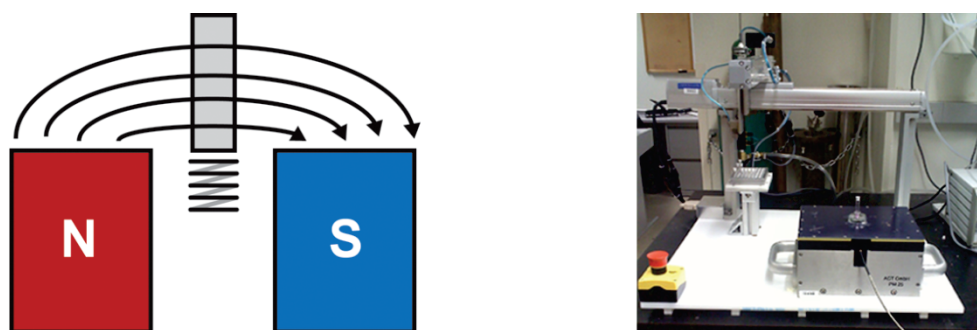
Figure 2.1. Schematic (left) of a single-sided magnet and picture (right) of the NMR-MOUSE with automation hardware (see Appendix F for further details on automation).
