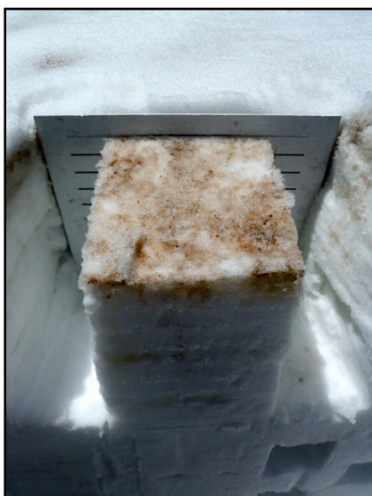
Figure 13 Rather than a continuous externally mixed layer of dust, like that which would result from artificial deposition, atmospheric deposition results in dust that is distributed amongst snow grains as internal and external mixtures, as exhibited in this DOS picture from SASP on May 10 th , 2013. The inability of SNICAR to capture absorption by such a heterogeneous mixture may account for NIR errors in the presence of heavy dust.
