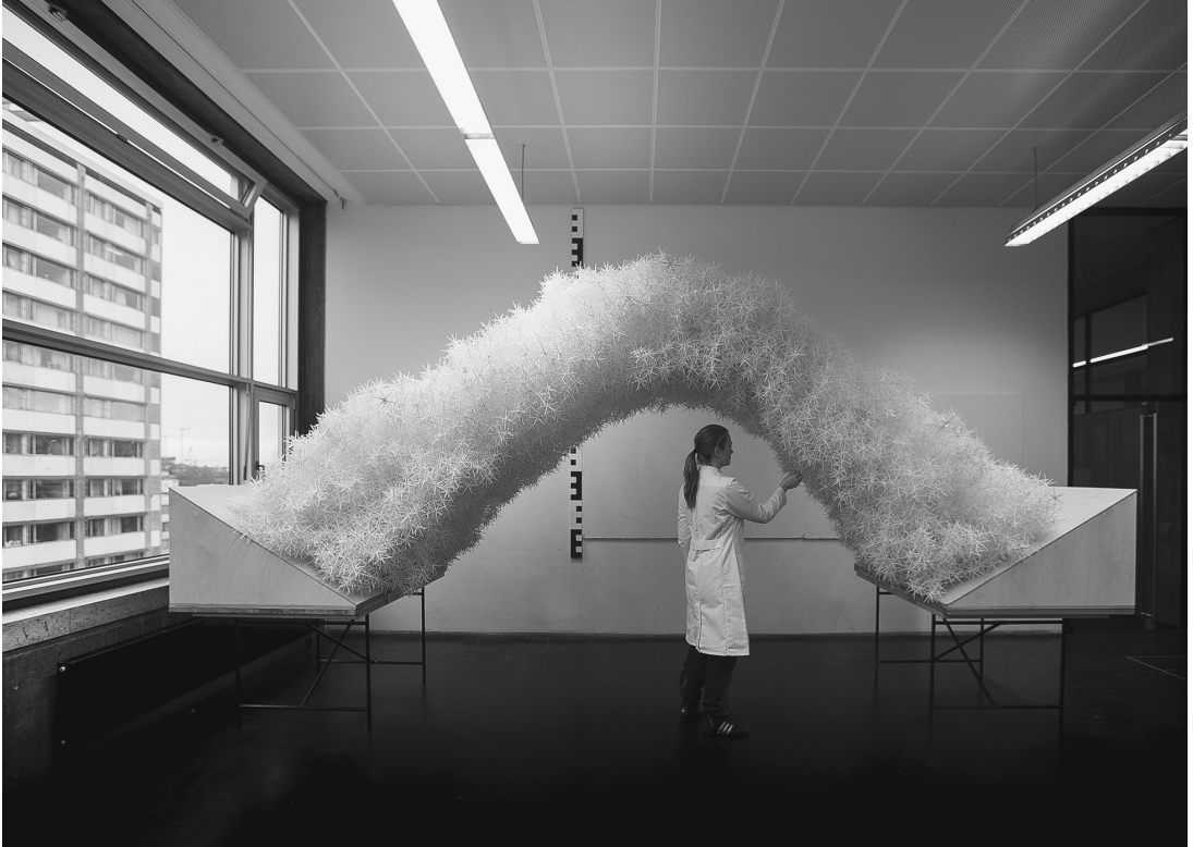
FIGURE 1.12. Aggregate Architectures , by Karola Dierichs, Institute for Computational Design, University of Stuttgart, 2014. By varying component morphologies, materials, or placement location, designers can create differentiated heterogeneous aggregate systems that perform to different capacities in different environments.
