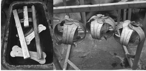
fig.8 - soaking birch plywood, component 004
