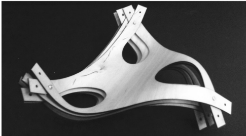
fig.9 - soaked birch plywood, component 007
