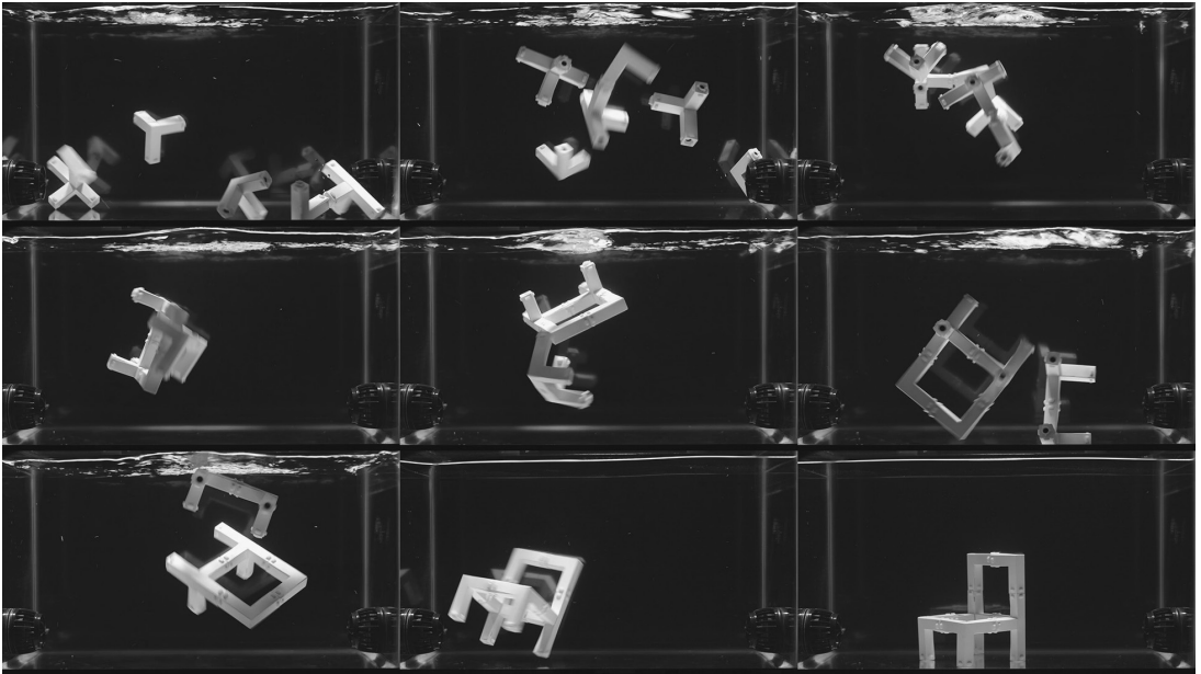
FIGURE 2.1. Fluid Assembly: Chair , by MIT's Self-Assembly Lab with Baily Zuniga, Carrie McKnelly, Athina Papadopoulou, and Skylar Tibbits in collaboration with Arthur Olson and Autodesk Inc., funded in part by MIT's International Design Center, 2014. This project entailed the design of uniquely differentiated parts that fit only one place in the final chair. Over seven hours, turbulent water in an aquarium jostled the parts until they joined together into the structure. Tibbits refers to this as "autonomous assembly" and states that it "points towards an opportunity to self-assemble arbitrarily complex differentiated structures from furniture to components, electronics/devices, or other unique structures."
