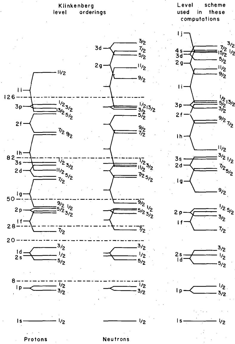
Fig. 1. Comparison of the Klinkenberg level ordering for shell-model states with the zero-deformation ordering employed in the present calculation.
