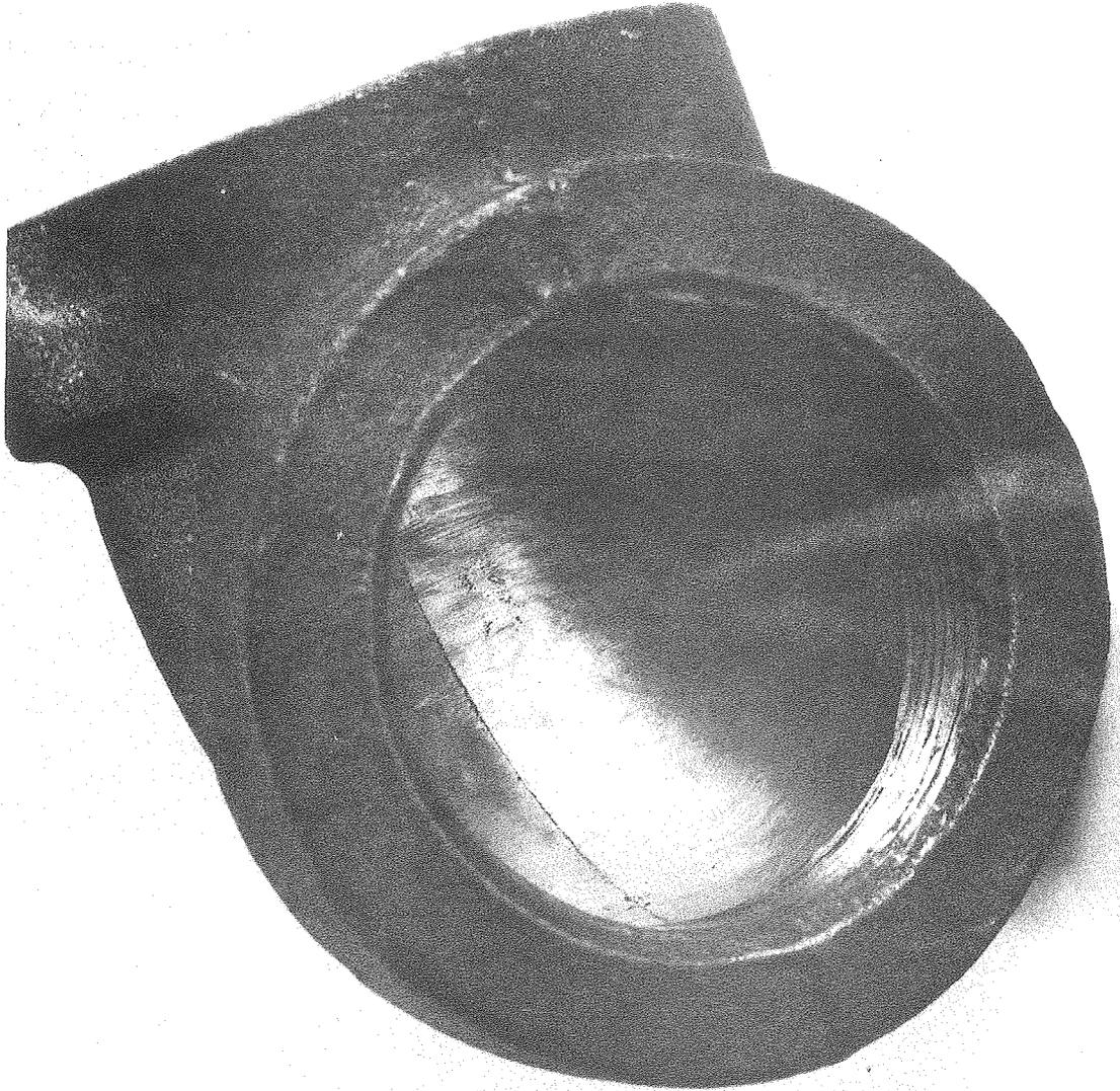
Figure 26. Ground elbow from 2" diameter pipe slurry loop.
