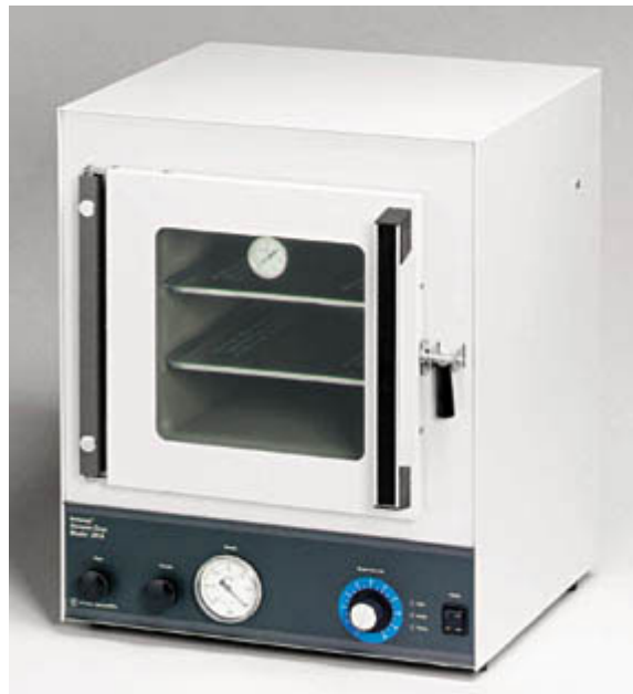
Fig. 2.5. The vacuum oven for degassing (Fisher scientific, Model 280A)
