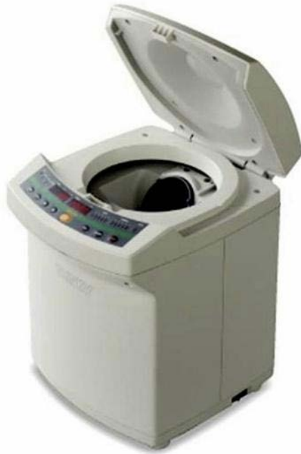
Fig. 2.4. The Thinky centrifuge mixer for silicone matrix and filler mixing
