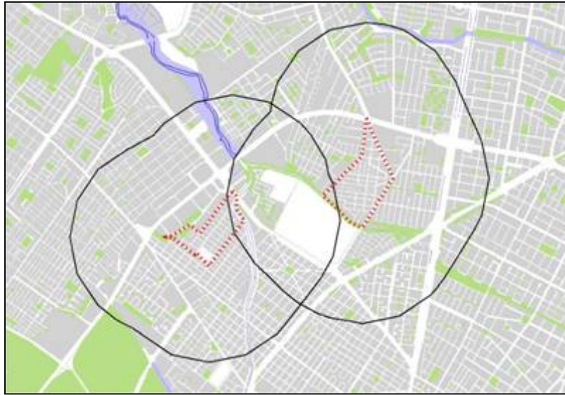
Figure 13. 500 meter Radii Around Sampled City Block for Measuring Walking Accessibility Levels in Bogotá
