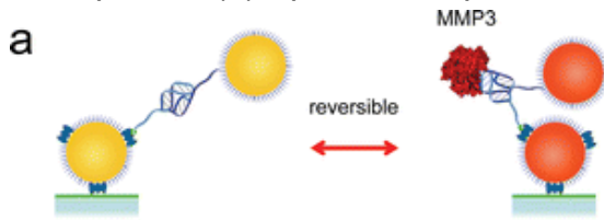
Figure 3. Aptamer-Au plasmon ruler binding to MMP3 molecules is reversible and specific. (a) Aptamer-Au plasmon ruler is immobilized with one nanoparticle bound to the glass surface using biotin-avidin chemistry. Peak wavelength of the plasmon resonance of an aptamer-Au plasmon ruler when alternately flushed with buffer containing 9 and 0 nM recombinant MMP3. The peak wavelength of the plasmon resonance increases (redshift) with addition of recombinant MMP3, indicating a decrease in the interparticle distance due to binding of recombinant MMP3 molecule to the aptamer-Au plasmon ruler. The peak wavelength of the plasmon resonance then decreases (blueshift) in the absence of recombinant MMP3, indicating an increase in the interparticle distance when the aptamer-Au plasmon ruler is unbound. Alternately flushing with buffer containing 9 and 0 nM recombinant MMP3 results in the peak wavelength that alternately redshifts and blueshifts, strongly suggesting that binding of MMP3 to the aptamer-Au plasmon ruler is reversible. (b) As a control, the peak wavelength of the plasmon resonance
