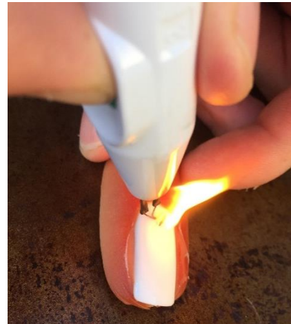
Figure. Acrylic nail igniting on simulated fingertip after trephination with an electrocautery pen.
