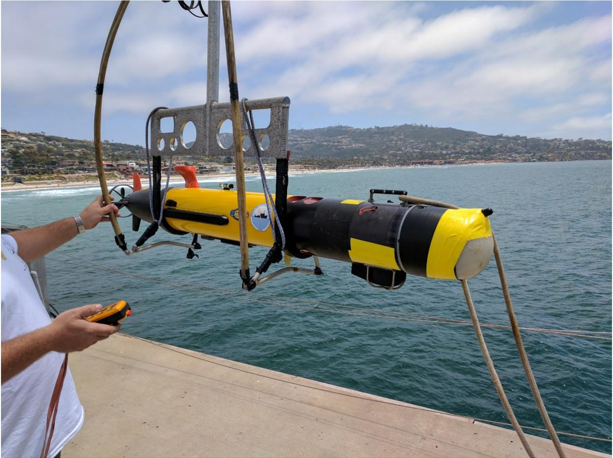
Figure 3.5: REMUS 100 vehicle used for this experiment, shown as it is being deployed. The hydrophone is visible at the vehicle nose. The modem hardware and passband recorder is incorporated within the vehicle's dry payload section (inside the yellow hull section).
