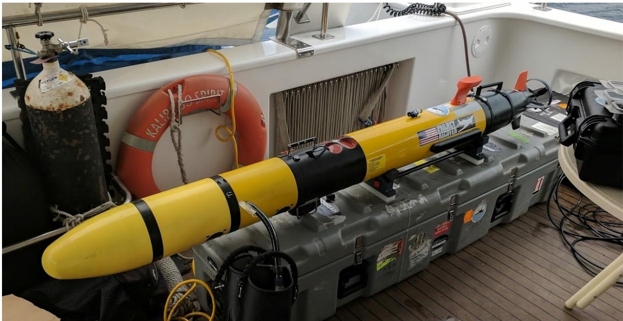
Figure 4.1: Sensor system in long housing attached to REMUS 100 AUV.
