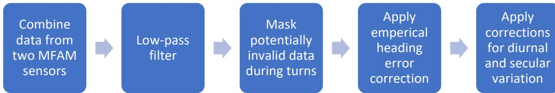
Figure 4.8: Flowchart showing summary of processing steps when using the AUV-based magnetometer to conduct geomagnetic surveys. This preserves low-frequency total field information.
