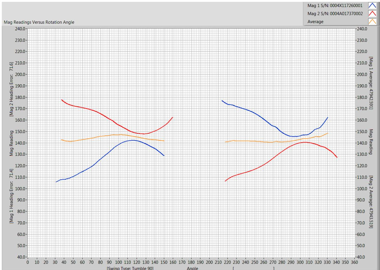
Figure 4.3: Intrinsic heading dependence of MFAM sensors. This corresponds to rotation in the azimuthal plane with the sensors mounted in a typical configuration on the AUV. The gaps in the traces correspond to the dead zone of the sensors, where no measurements are possible. Measured values are in nanoTeslas (nT). Figure courtesy Geometrics, Inc. Used with permission.
