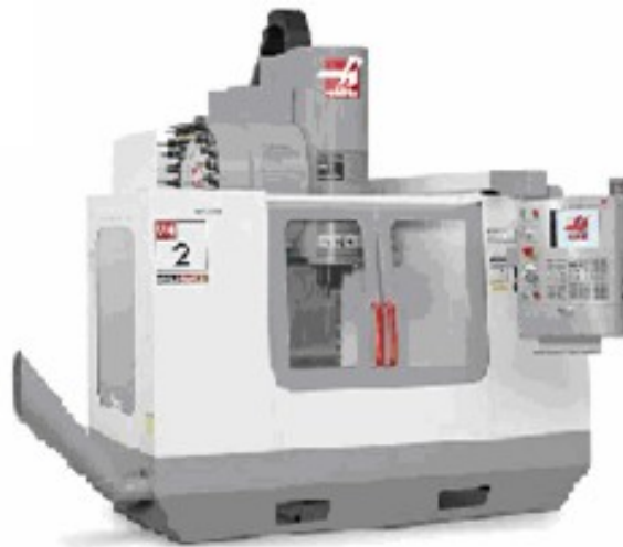
Figure 4.28: Computer numerical control (CNC) milling machine with 3-axis control, tool changer and control panel (Haas Automation Inc, 2013)
