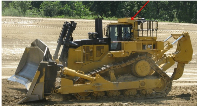
Figure 4.7: Caterpillar Inc. D11 track type tractor showing the canopy component placement as part of the larger assembly/finished product, the D11 is the largest in the D series track type tractors manufactured by Caterpillar.
