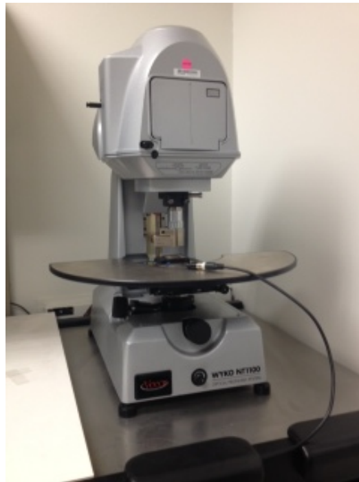
Figure 2.7: Image of the WYKO interferometer used for testing the deformable mirrors
