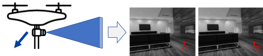
Figure 1.2: Schematic showing potential application of the approach with a drone. Drone captures images, Fourier pre-processor is applied computationally to pairs of images, and a small brain neural network infers position as illustrated in Fig. 1.1.
