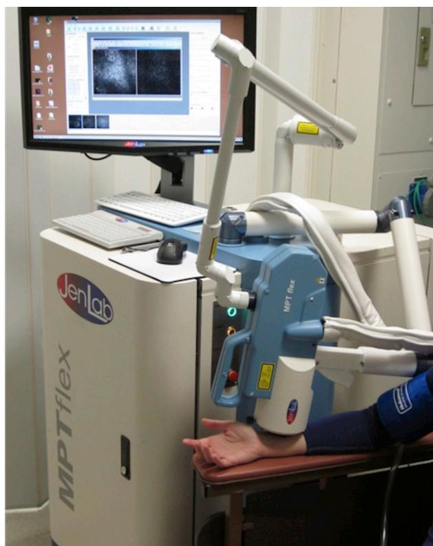
FIGURE 1 MPM-based clinical tomograph (MPTflex) during the occlusion experiment.
