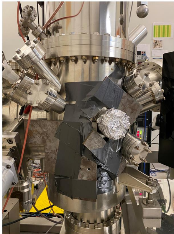
Figure 2.8 STM head drift correction. A photograph of the STM chamber with several iron plates attached to it, which can reduce the STM head drift when a magnetic field is applied.
