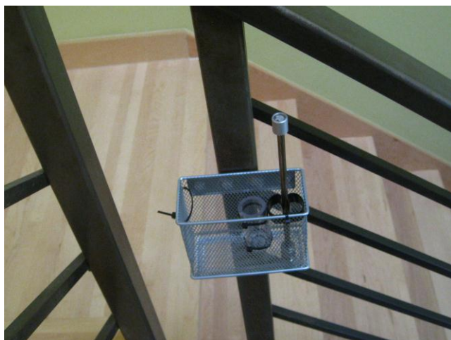
Figure 9 Example of Passive Sampling Tube Installed on Stair Rail with Wire Mesh Basket, Project 0902
