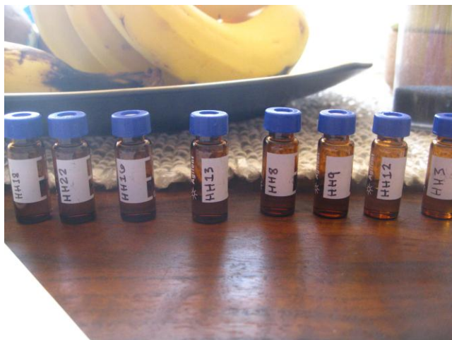
Figure 8 Eight Passive Emitter Tubes with Tracer Gas, Project 0902
