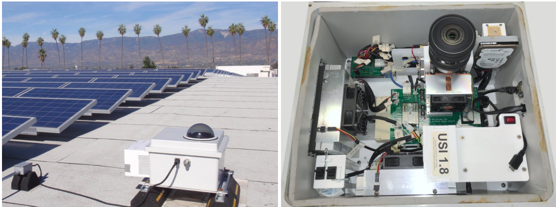
Figure 1.2: Photographs of UC San Diego Sky Imager (USI) hardware
