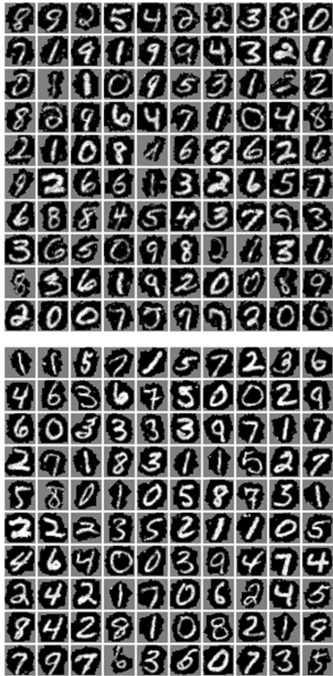
Figure 3.4: Synthesized images using transferred D-Patch dictionaries. The top half shows 100 reconstructed MNIST images synthesized from a dictionary learned on USPS. The bottom half shows the other way around.
