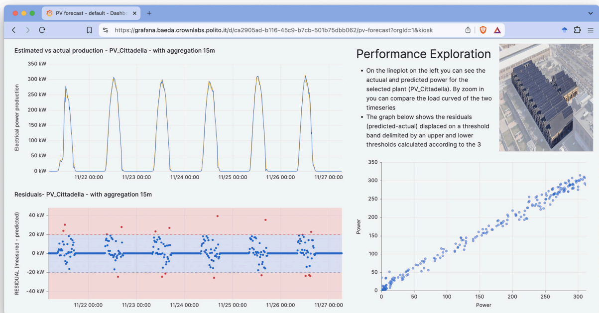
Fig. 9. Screenshot of the online Campus dashboard used to visualize the results of the LSTM model during the validation period.
