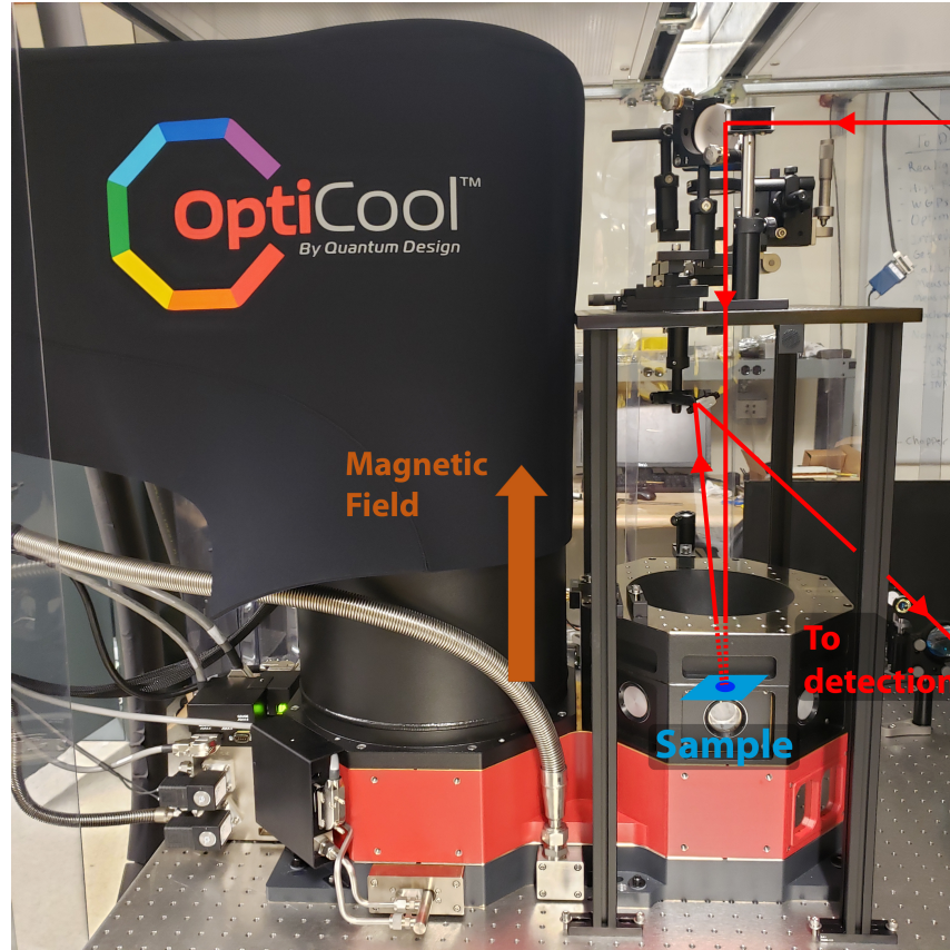
Figure 3.2: The experimental setup for magnetic field-dependent measurements. The system is a Quantum Design OptiCool closed-loop cryostat. Measurements are performed in reflection, coupled into the top of the cryostat with a raised periscope assembly. The magnetic field is out of plane. Transmission measurements through the side windows are also possible.
