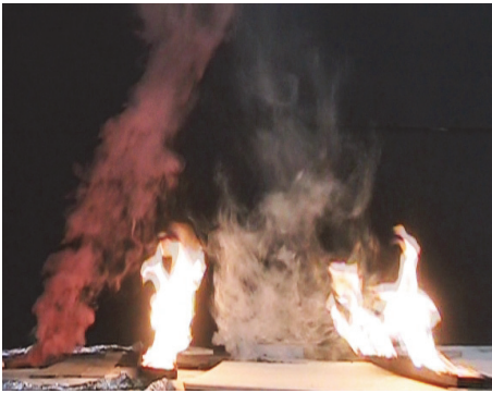
FIGURE 8: Use of smoke cartridges for flow field visualization. Exaggerated flame angle on right is fictitious, due to perspective distortion (figure is cropped; camera is actually centered on left fire).
