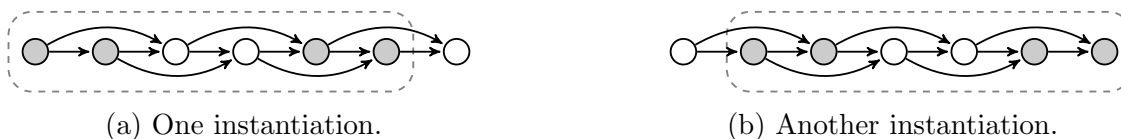
Figure 8.2: Two instantiations of a structural motif in a directed chain of length seven. The motif consists of two consecutive variables and their Markov blanket of four neighboring variables. Each instantiation is separated into block proposed variables B_i (white) and conditioning variables C_i (shaded).
