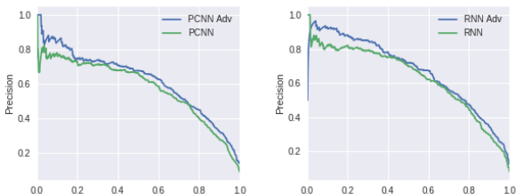
Figure 7.3: PR curves for PCNN (left) and RNN (right) on the UW dataset with (blue) and without (green) adversarial training.
