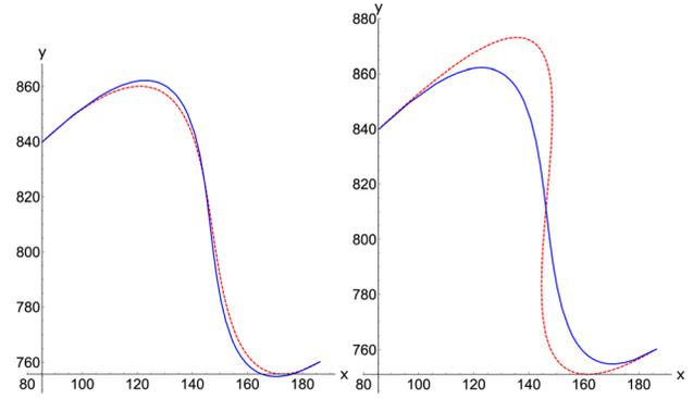
**Fig. 2** Cubic trigonometric Bezier curve with  $\lambda = -0.5$  in dashed compared to the cubic Bezier curve in solid and cubic trigonometric Bezier curve with  $\lambda = 0.5$  in dashed compared to the cubic Bezier curve in solid
