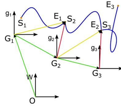
**Fig. 5 An example showing the vectors used to calculate the ground pivots  $\mathbf{G}_j$**
