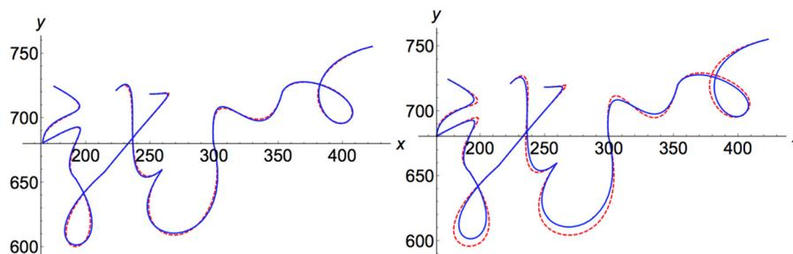
Fig. 12 The cubic trigonometric Bezier curves with  $\lambda = -0.5$  (dashed) fit the cubic Bezier curves (solid), and the cubic trigonometric Bezier curves with  $\lambda = 0.01$  (dashed) vary from the cubic Bezier curves (solid)
