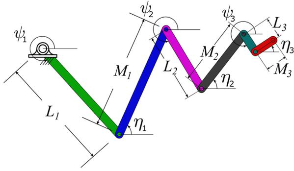
**Fig. 1** The six-link coupled serial chain is constructed so that each sequence of two links,  $L_k$  and  $M_k$ , rotates in opposite directions at a multiple  $k$  of the base joint rate. The phase angles,  $\psi_k$  and  $\eta_k$ , define the initial configuration of the trigonometric Bezier curve.
