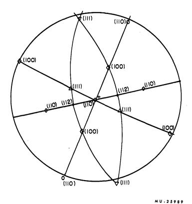
Fig. 8. A stereographic projection of a cut single-crystal filament oriented with a (110) plane the surface normal to the long axis.
