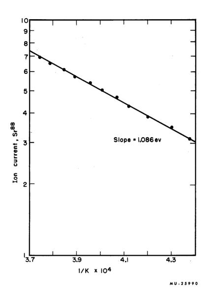
Fig. 10. Typical Saha-Langmuir plot of the ion current against reciprocal filament temperatures for strontium on "bulk" tungsten.
