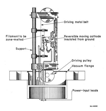
Fig. 1. Equipment used to strain-anneal tungsten filaments.
