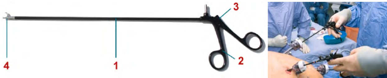
Figure 2.1: Left: A traditional laparoscopic tool consists of a stiff shaft (1) connected to a gripper (2) that pivots around a hinge (3); this closing motion is translated to an end-effector (4) that can be scissors, grippers, retractors, etc. Right: Laparoscopic tools inserted through cannulae in the abdomen.
