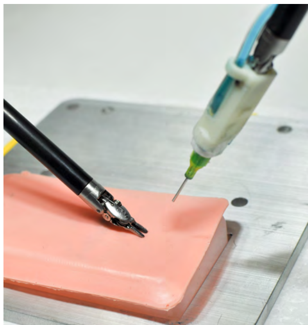
Figure 4.1: This delivery instrument can provide controlled local injections of mesenchymal stem cells to hard-to-reach areas within body cavities using a single-use disposable needle tip.
