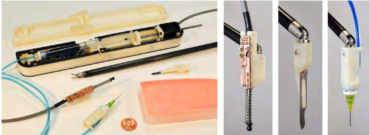
Figure 5.7: The suite of surgical tools created for increased autonomy in Robotic Minimally Invasive Surgery. At Left: The surgical adhesive injector and other tools shown with a US penny for scale. At Right: Tools mounted on a daVinci surgical retractor (featuring PALP, a scalpel, and FLIP)
