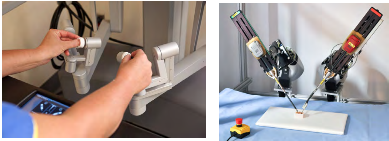
(a) Master exoskeleton with two 7 DOF manipulators. (b) Surgical arms controlled by telepresence. Figure 2.3: The da Vinci Robotic Surgical Assistant (RSA) consists of a master exoskeleton and two slave arms. The da Vinci Robotic Surgical Assistant is controlled by a surgeon's hand movements.
