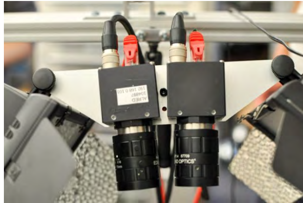
Figure 6.4: Two Allied Vision Technologies Prosilica GC1290C were used to support stereoscopic vision during suturing experiments. These cameras were chosen because they can be set up with a larger baseline (distance between optics) than standard endoscopes.
