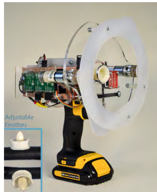
Figure 1.3: The DATE is designed to interface with inexpensive passive irrigation emitters distributed in a field to alleviate the financial burden placed on farmers in California’s drought.
