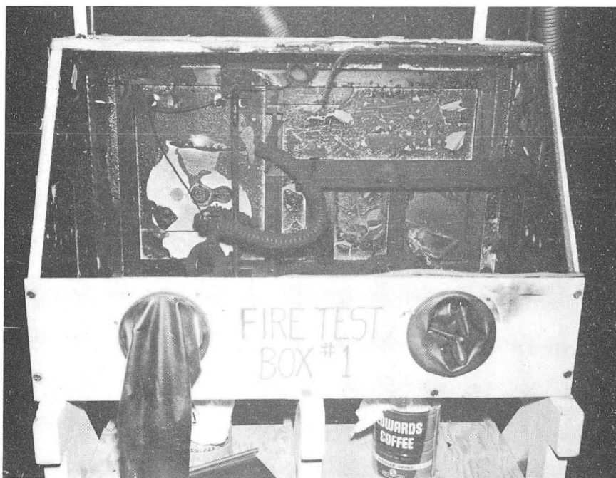
Fig. 4. Standard plywood box after internal fire. (Health Pro 812)
