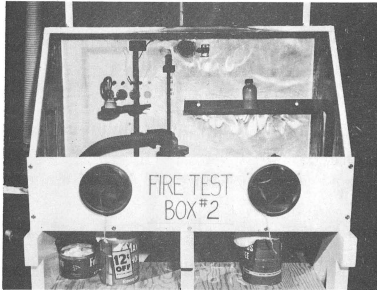
Fig. 5. Asbestos-millboard box after internal fire. (Health Pro 803)
