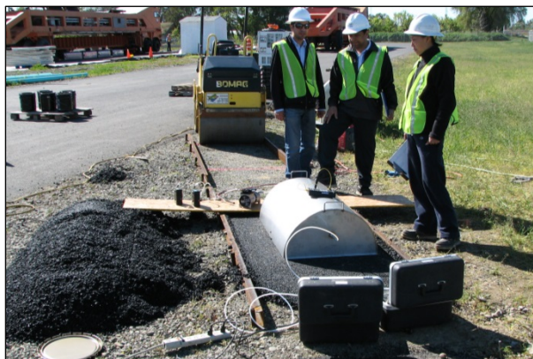
Figure 3.5: Test section compacting prior to sampling.
