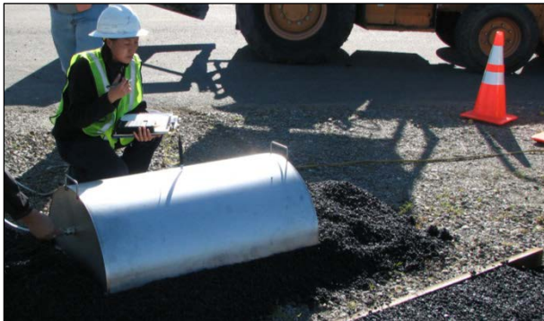
Figure 3.4: Stage 2 sampling on loose mix.
