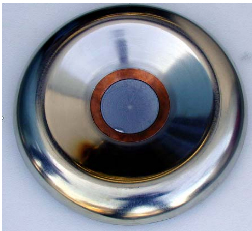
Fig. 7. A photograph of a 10 cm diameter aluminosilicate emitter with the Pierce electrode.
