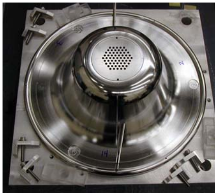
Fig. 14. Photograph of an electrode in the full-gradient accelerator showing the 61-beamlet aperture array.
