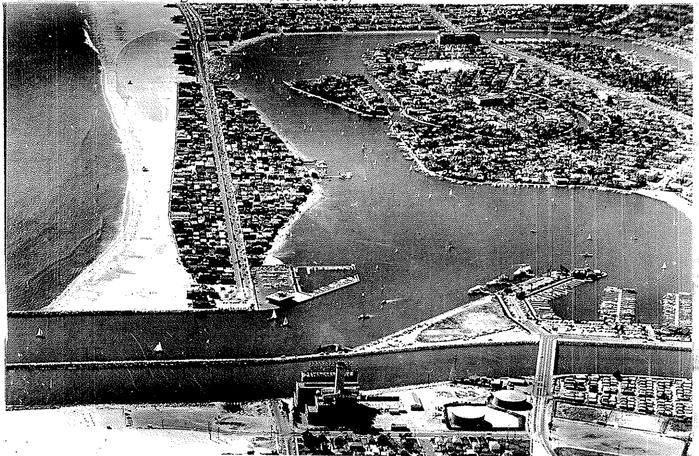
Figure 7. Alamitos Bay, California, August 1964. Oblique Aerial Photo Looking Northwesternly Over Bay; San Gabriel River Channel/Mouth and Bay Entrance, and Three Contiguous Jetties at Bottom; Peninsula at Left. (From USACE, Los Angeles District, 1966/1967)
