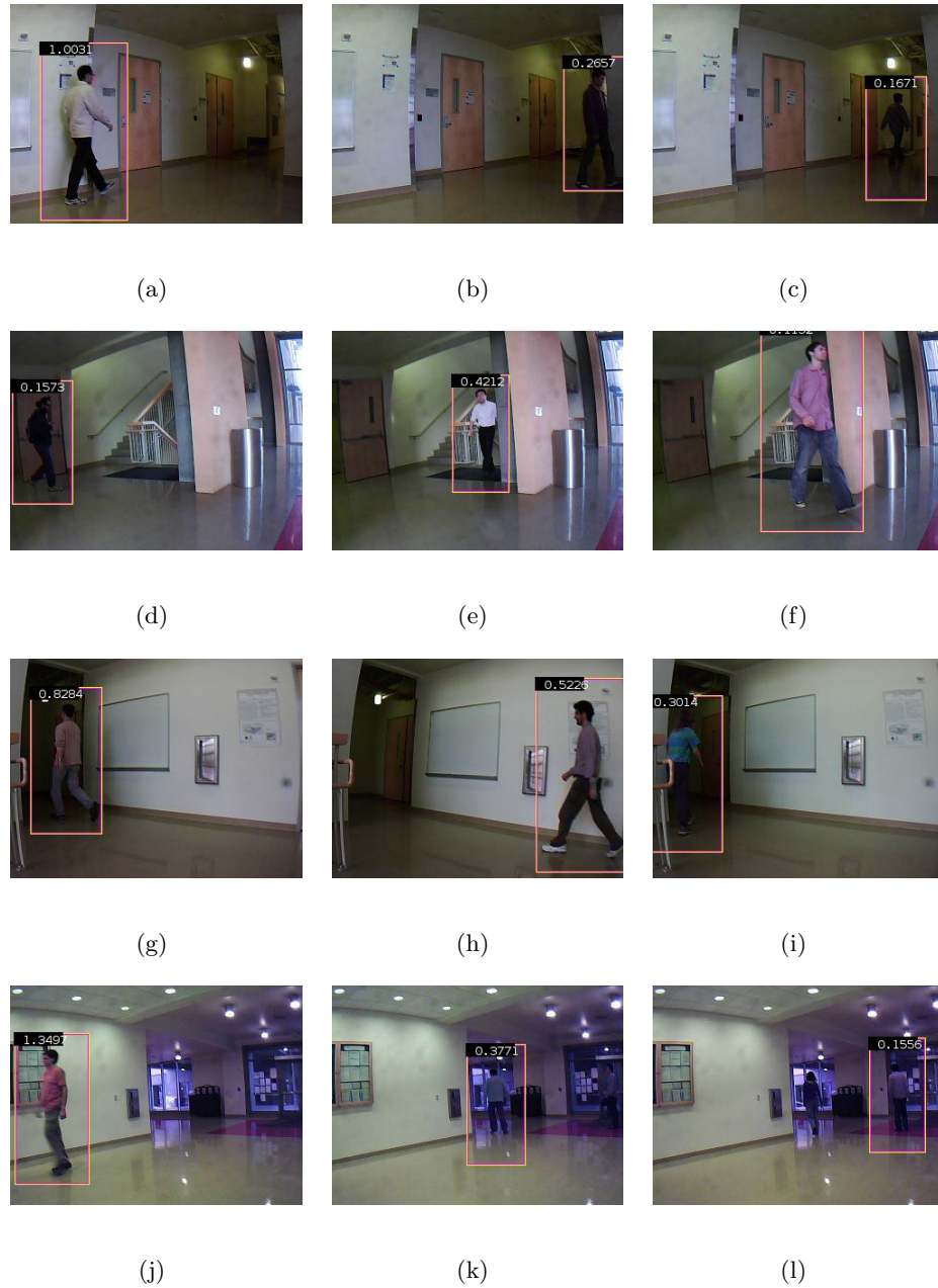
Figure 4.4: Human detection results. Images (a)-(l) are shots at states Z_1 to Z_{12} , respectively. We can see from the images that detected subjects are of different viewpoints, different size and under different lighting conditions, which makes the object association problem more difficult. The coordinates of the bounding box could help in turn identify the entering/leaving state of the subjects.
