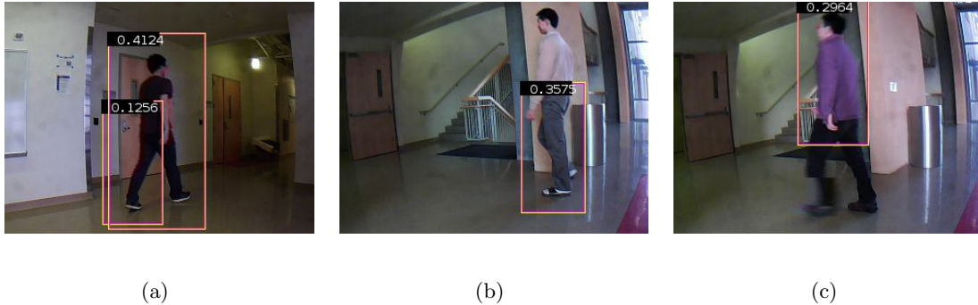
Figure 4.5: Some false positive from our HOG-based detector. Most of the false positives can be removed using prior spatial knowledge. (a) One bounding box is embedded in the other. (b) The y_{min} coordinate of the bounding box is too large (i.e., the detected person is too small). (c) The y_{max} coordinate of the bounding box is too small (i.e., the detected person is not on the floor).
