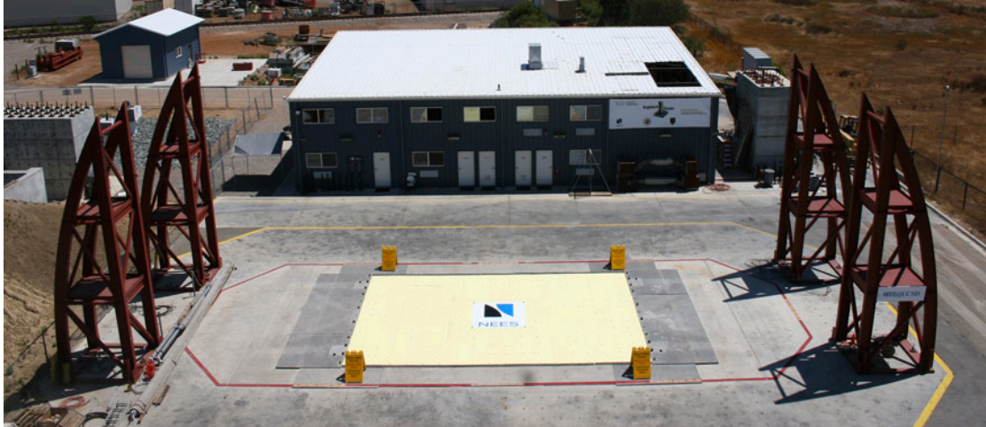
Figure 2.1. UCSD Large High-Performance Outdoor Shake Table (source: NEES, 2014).
