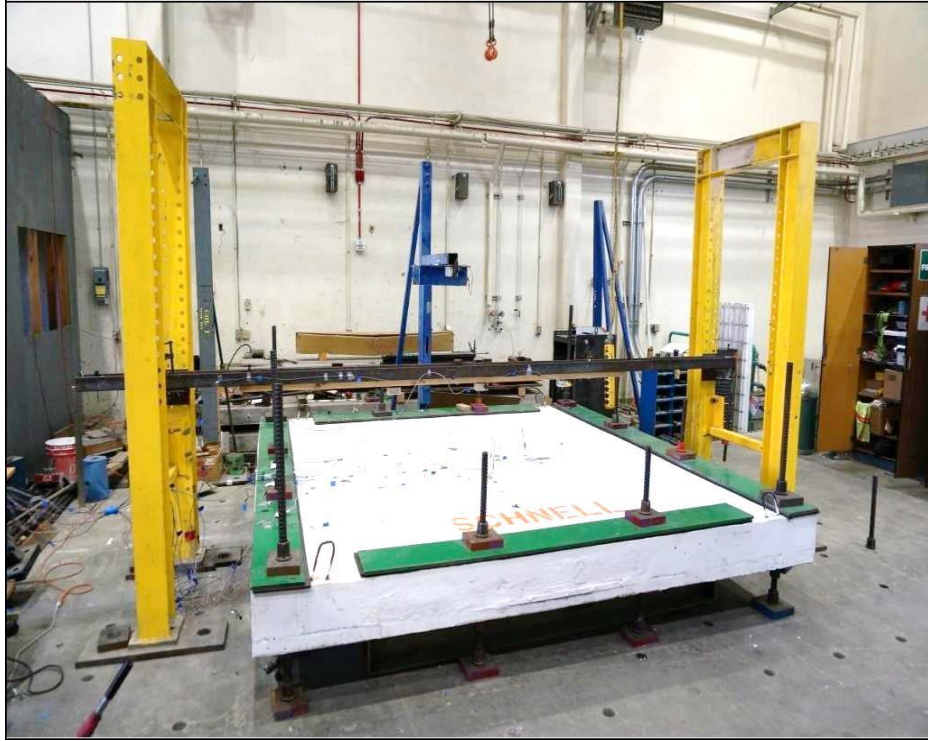
Figure (3.30): Experimental Setup for Sandwich Slabs A and B
