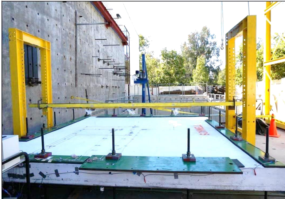
Figure (3.31): Experimental Setup for Sandwich Slab C
