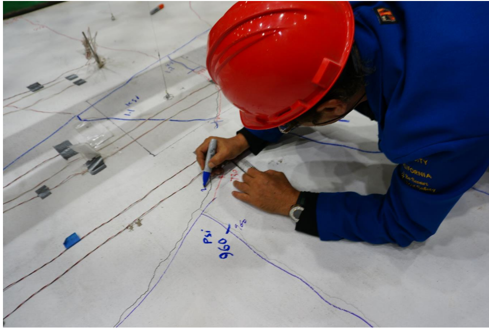
Figure (3.43): Cracks were Monitored, Recorded and Analyzed throughout the Test
