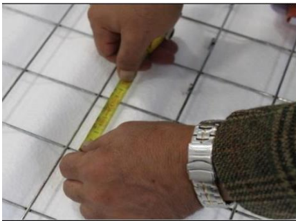
Figure (3.5): Measurement of Welded Wire Mesh
