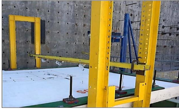
Figure (3.35): Setup Showing Steel Channel Placed Between Steel Frames.
