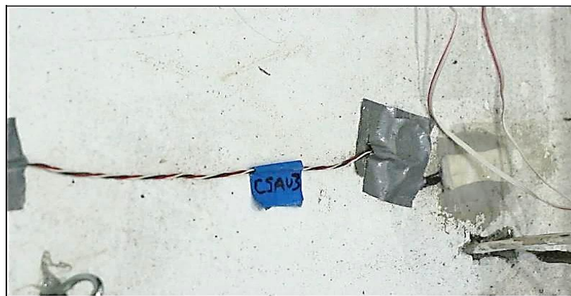
Figure (3.18): Strain Gauge on Mortar Surface.
