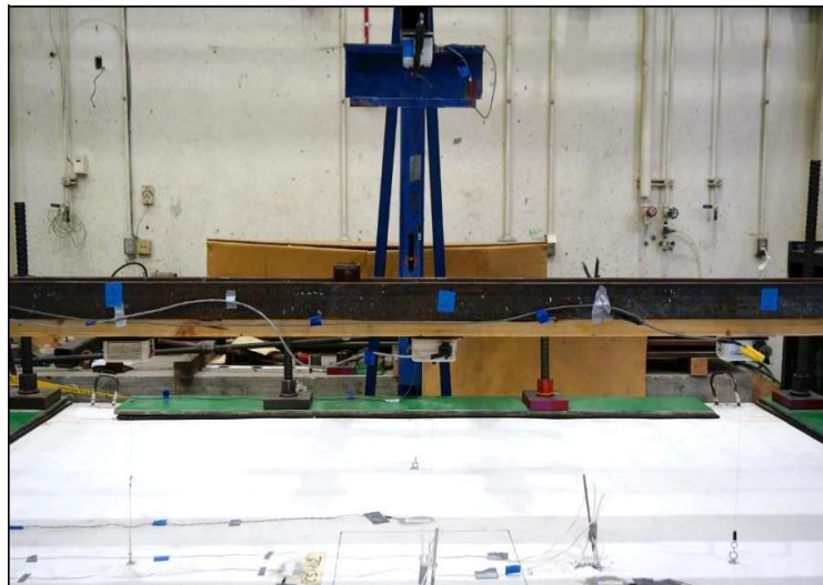
Figure (3.36): Set Up Showing String Potentiometers SP1, SP2, and SP3 Attached to the Sandwich Slab Top Surface
