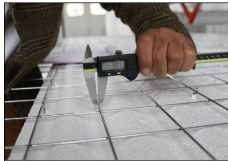
Figure (3.6): Measurement of Diameters of WWF Wires
