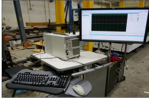
Figure (3.20): Data Acquisition System to Record Experimental Data
