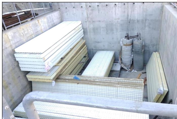
Figure (3.4): Test Specimens prior to Mortar Application
