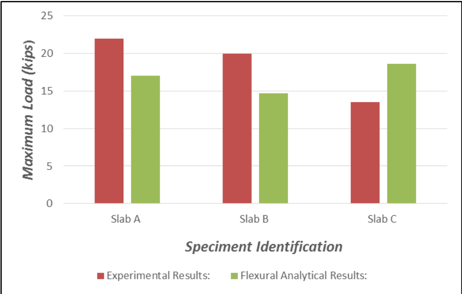
Figure(4.6): Comparison of Experimental Load Capacity with Predicted Load Capacity in Flexure.
