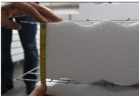
Figure (3.7): Measurement of Thickness of EPS between WWF
