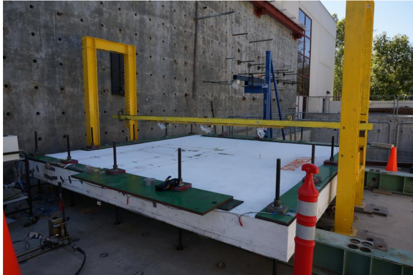
Figure (3.53): Test Setup for Sandwich Slab Specimen C
