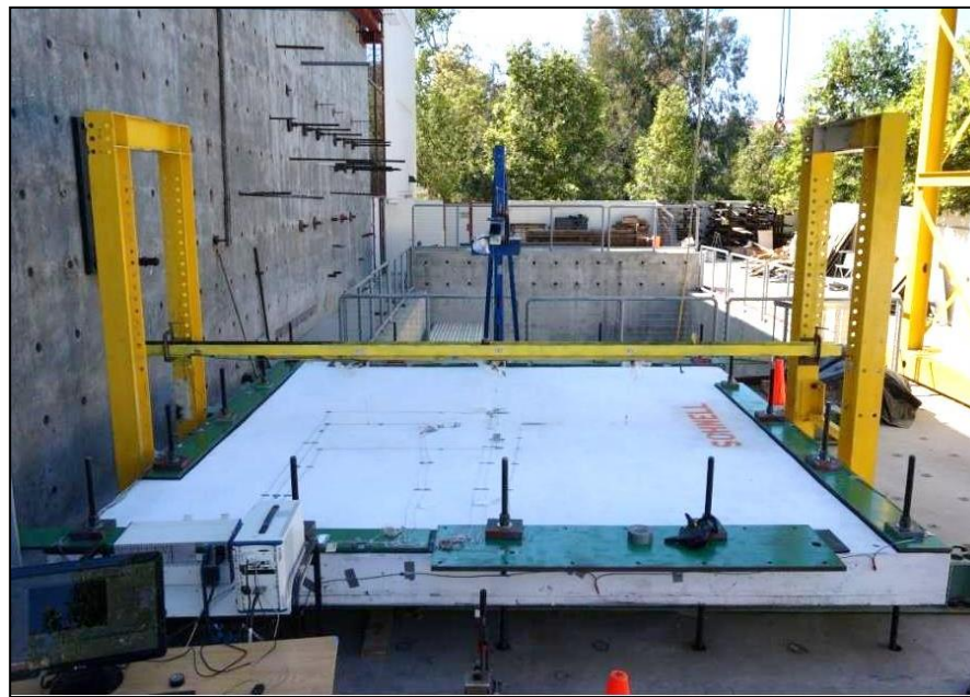
Figure (3.39): Experimental Setup for Sandwich Slab C
