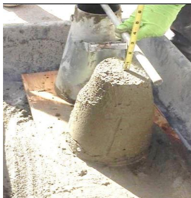
Figure (3.9): Measurement of Slump at UCI SETH Laboratory
