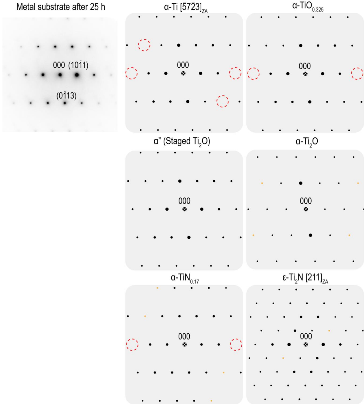
Figure 4.8. Experimental SAED from the metal substrate of titanium exposed to gettered Ar at 800°C for 25 h and fast-cooled. Indices shown correspond to \alpha -Ti along a [\bar{5}\bar{7}\bar{2}\bar{3}]_{ZA} zone axis. Yellow spots represent forbidden or double diffraction spots. Schematics of simulated suboxide, solid solution, and nitride SAED patterns are shown with gray backgrounds.
