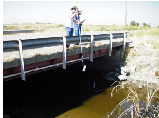
DO-46 Mud Slough at Gun Club Sampling crew deploying Sonde and taking water samples from bridge.
