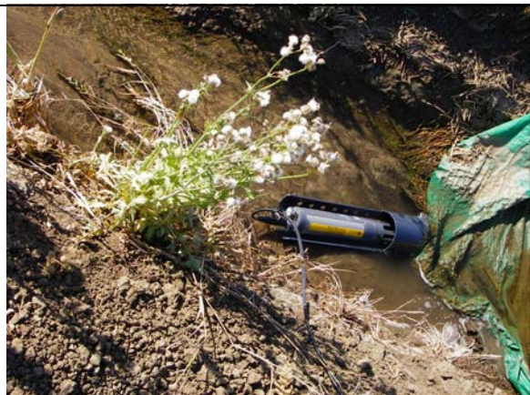
DO-101 WFP-UD-IN The Sonde is in the un-vegetated ditch with a custom made shield to protect it from the plants in the ditch.
