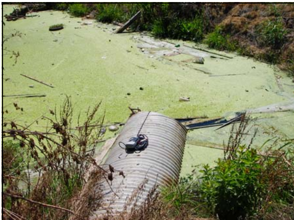
DO-88 Ramona Drain at Apricot Ave. Sonde deployed off of pipe. The site has large amounts of duck weed and other aquatic vegetation.
