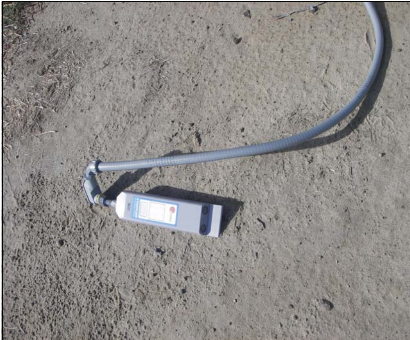
Starflow Doppler flow meter Picture of Sontek Doppler flow meter with protective tubing around cord. The Starflow is put on the bottom of the channel to measure flow.
