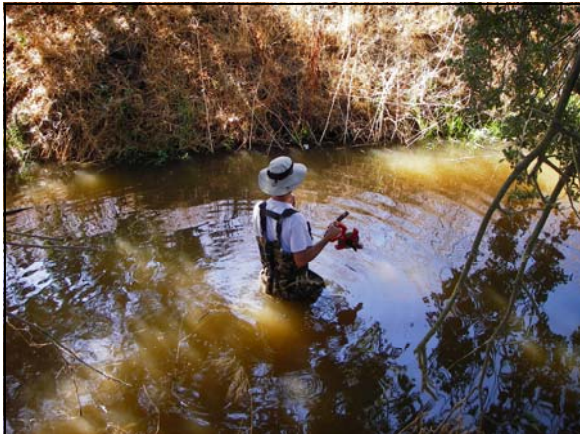
DO-86 Ramona Drain at Apple Ave. Jeremy Hanlon performing a stream rating across Ramona Drain.
