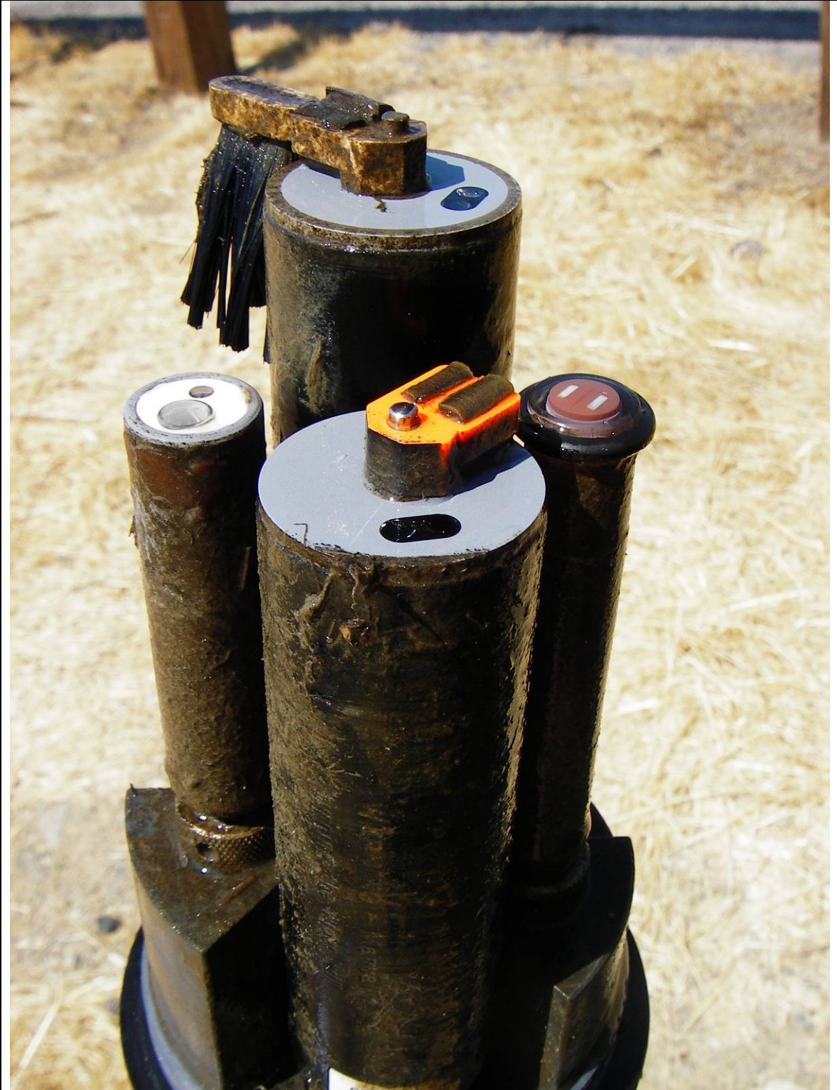
Fig. 5 Sonde at end of 2 week deployment showing effectiveness of wipers
