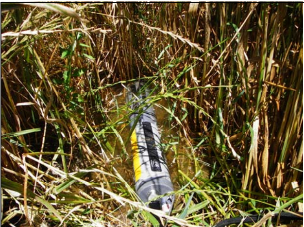
Vegetated Ditch Sonde in vegetated ditch. Water barely covered the sensors.
