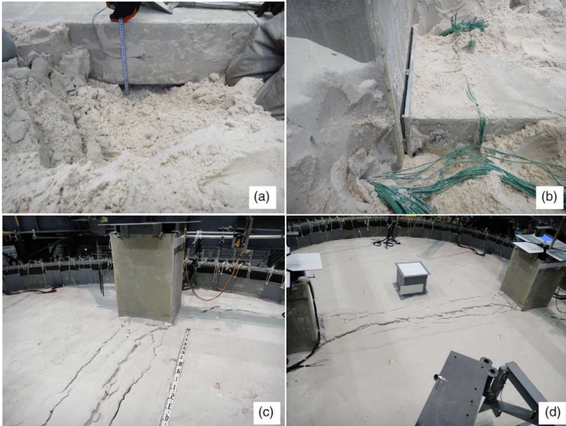
Figure 4.5. Observed damage after the 80% Takatori motion: (a) settlement beneath the cut-and-cover tunnel (photo taken after excavation), (b) failed resin bolts on the rigid joint, and (c, d) cracks at the ground surface parallel to the buried cut-and-cover tunnel
