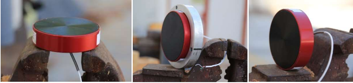
Figure 3.3. Photo of pressure cell (left and middle), and pressure cell with adapter ring (right)
