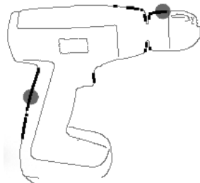
Figure 5.2: Example of the Image Processing component, showing the edge detection (grey pixels), pixels with a 90% probability or higher of being good grasping points (black pixels), and the two points selected for the regrasp configuration (circles).
