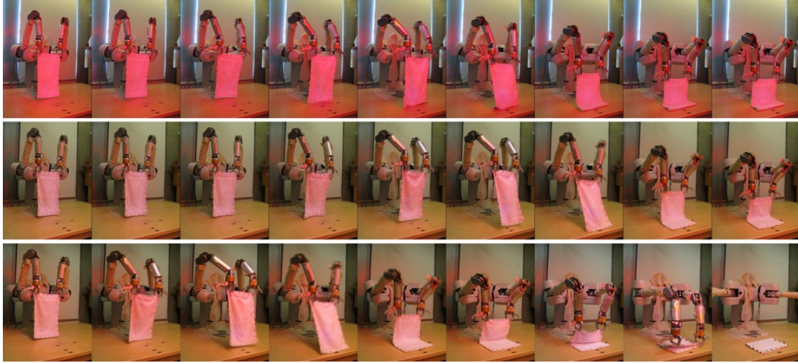
Figure 6.13: Trials producing rewards of 0.57391 (top) and 0.93905 (middle), along with final folding motion (bottom).
