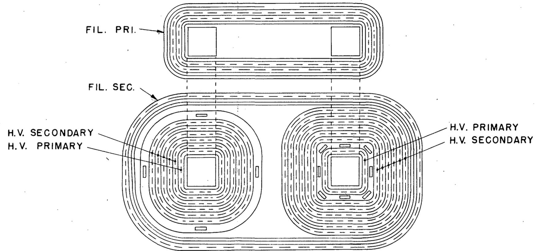
CROSS SECTION OF WINDINGS & INSULATION
