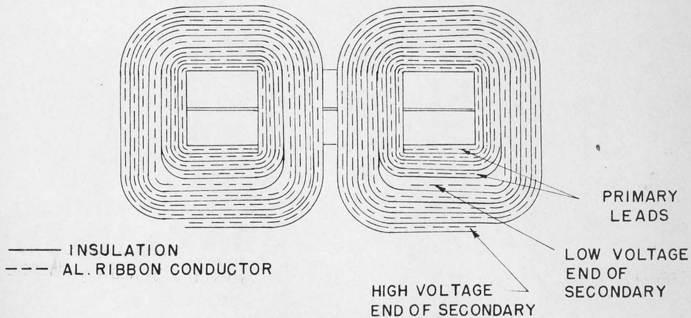
METHOD OF WINDING FOIL-PAPER HIGH VOLTAGE PULSE TRANSFORMERS.
