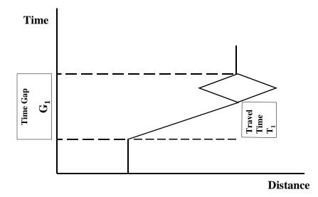
FIGURE 3 Prism Volume as Measurement of Accessibility
