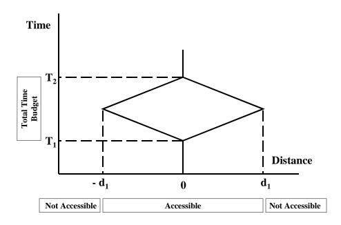
FIGURE 1 The Basic Form of a Space-Time Prism
