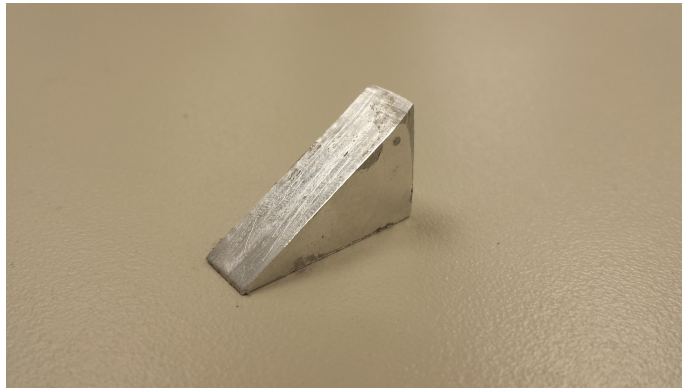
Figure 4.11: Right-angled triangular prism fabricated from aluminum with smallest angle of 30 degrees. The hypotenuse of this piece is 32.4 mm.
