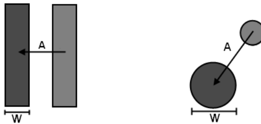
Figure 5.1: Using an applet, sequences of rectangular and circular targets are presented to users, where target distance A and width W can remain constant (homogeneous) or vary (heterogeneous) after every click.
