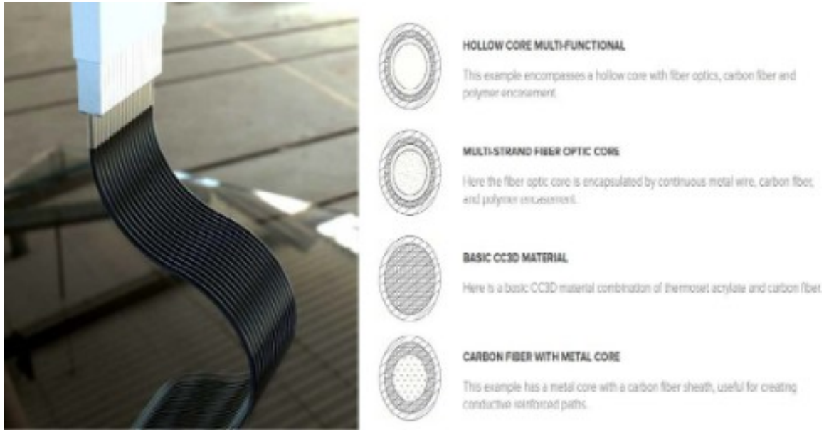
Figure 1.6: Functional 3D printing with 16 channel nozzles and materials.
