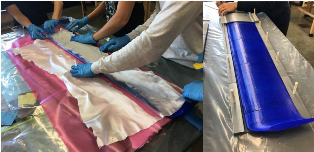
Figure 3.29: Layup (Left), and Wing in Mold (Right)
