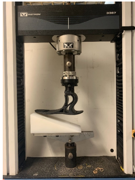
Figure 7.3: LIMBER ankle-foot mounted on the Instron testing machine ready for toe side static and cyclic testing.
