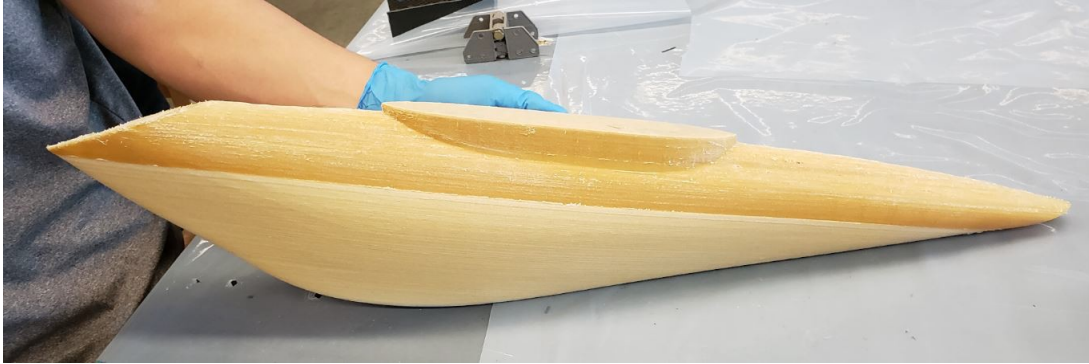
Figure 3.37: Final 3D printed Fuselage Mold.
