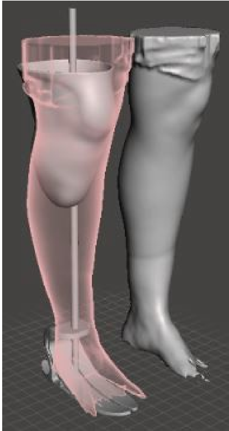
Figure 6.5: Sound Leg Model and Mirrored Leg Combined with Residual Limb, used to size and align components for the generation of a monocoque design.
