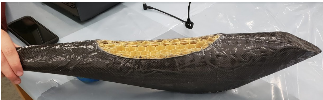
Figure 3.38: Final Carbon Fiber Reinforced Polymer Fuselage, mold has not been dissolved yet.
