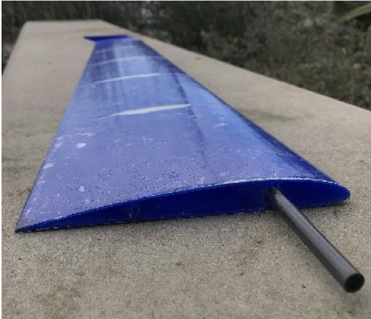
Figure 3.30: Final Fiber Reinforced 3D Printed Wing
