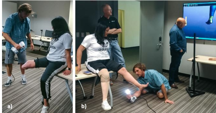
Figure 6.4: Laser Scanning workflow: a) while activating the scanning device the residual limb is scanned by moving the scanner around the region of interest. b) In a similar matter the healthy leg was scanned.
