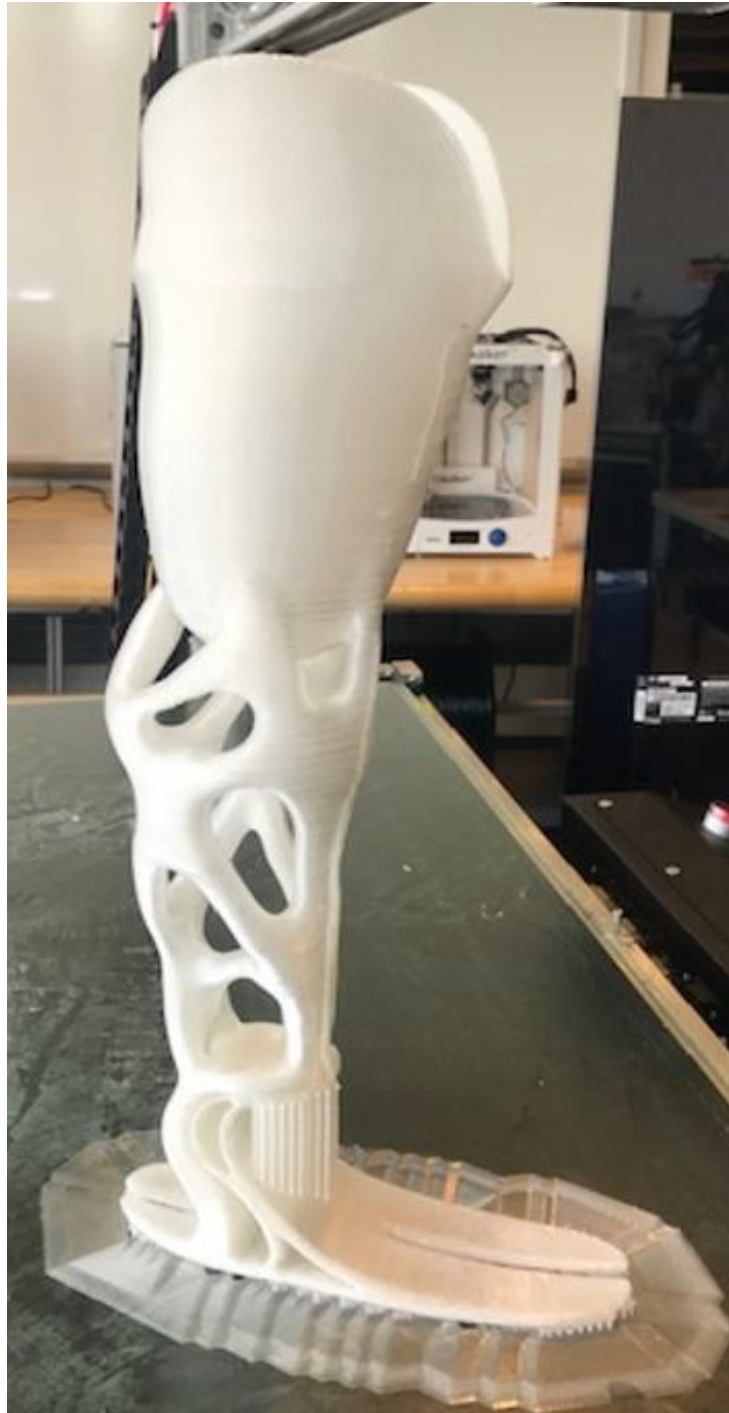
Figure 6.17: Final version of full-scale LIMBER 3D Printed Prosthesis Monocoque Version.
