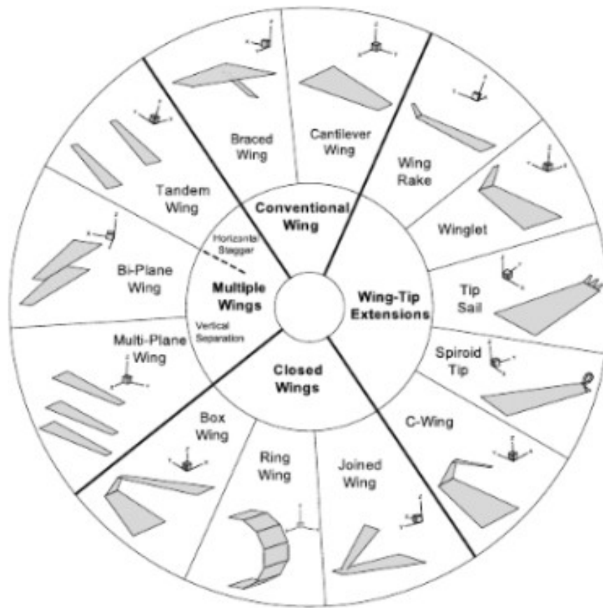
Figure 2.2: Different Non-planar Wing Designs. Box-Wings are a Member of the Closed Non-Planar Wing Family.
