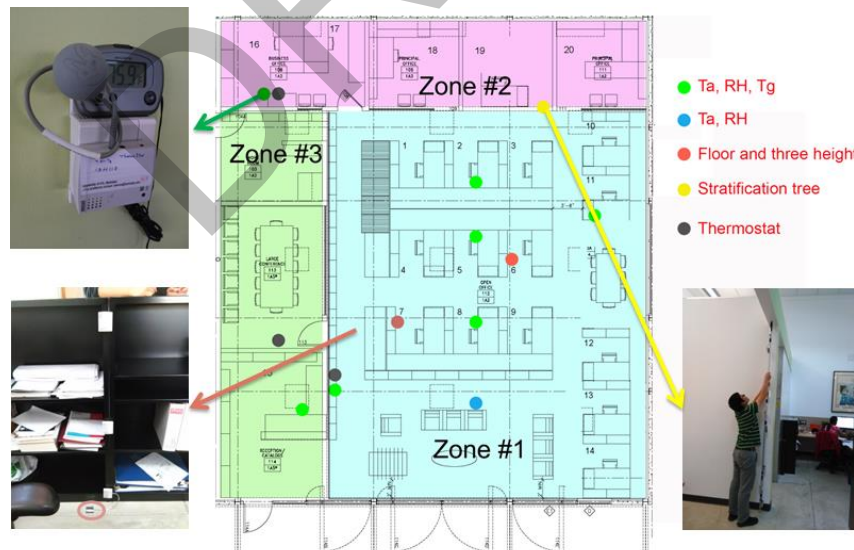
Figure 4.4. Measurement devices and locations at Integral Group office
