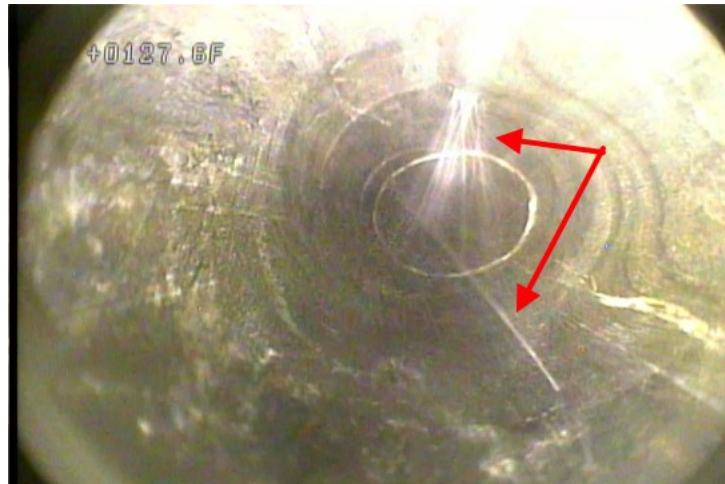
Figure 4. E1. Water jetting into borehole E1-P (see arrows).
