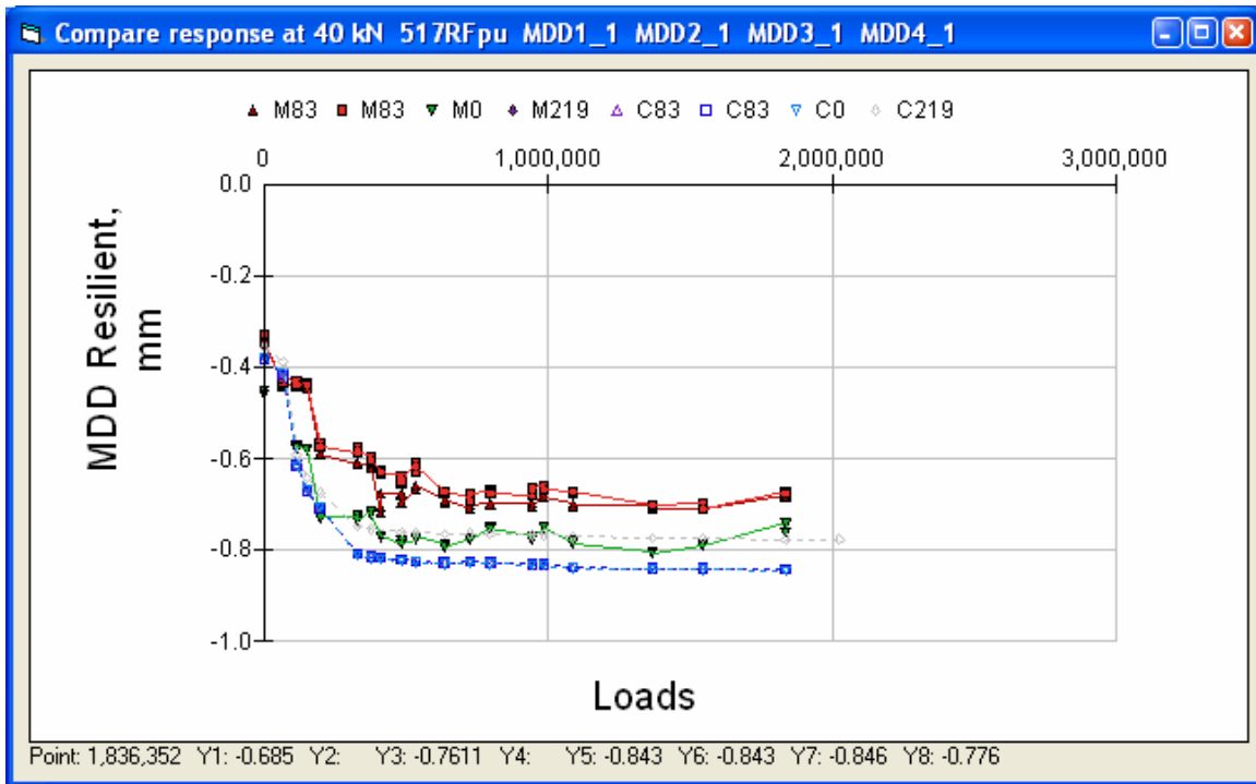
Figure 81. Section 517RF 40 kN deflection of top modules.
