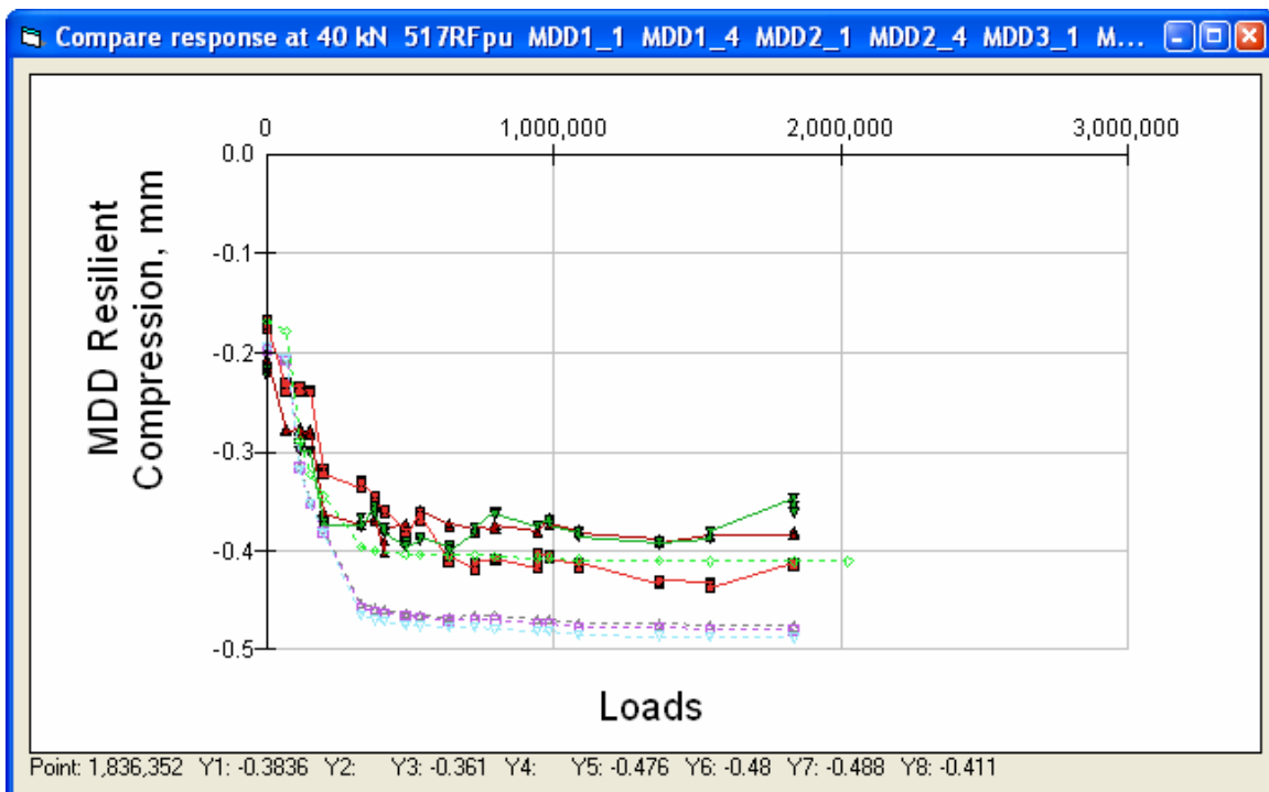
Figure 82. Section 517RF 40 kN compression of pavement layers.
