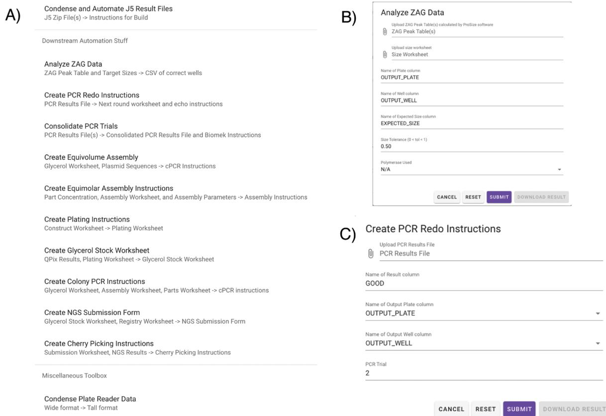
**Figure 2.** DNAda core features. (A) DNAda contains numerous functions that automatically create customized liquid handler instructions given design files and result files. (B) An example intermediate workflow involves analyzing uploaded PCR result data from the ZAG. (C) DNAda can then use that uploaded PCR data in order to generate automated redo PCR instructions for the failed reactions.
