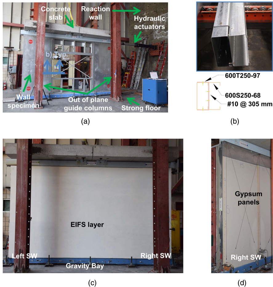
Fig. 1. (a) Specimen SWWS-2 as installed in test setup; (b) jamb stud built-up section used around window opening; (c) front view of exterior face of Specimen SGG-2F; and (d) isometric view of interior face of Specimen SGG-2F.
