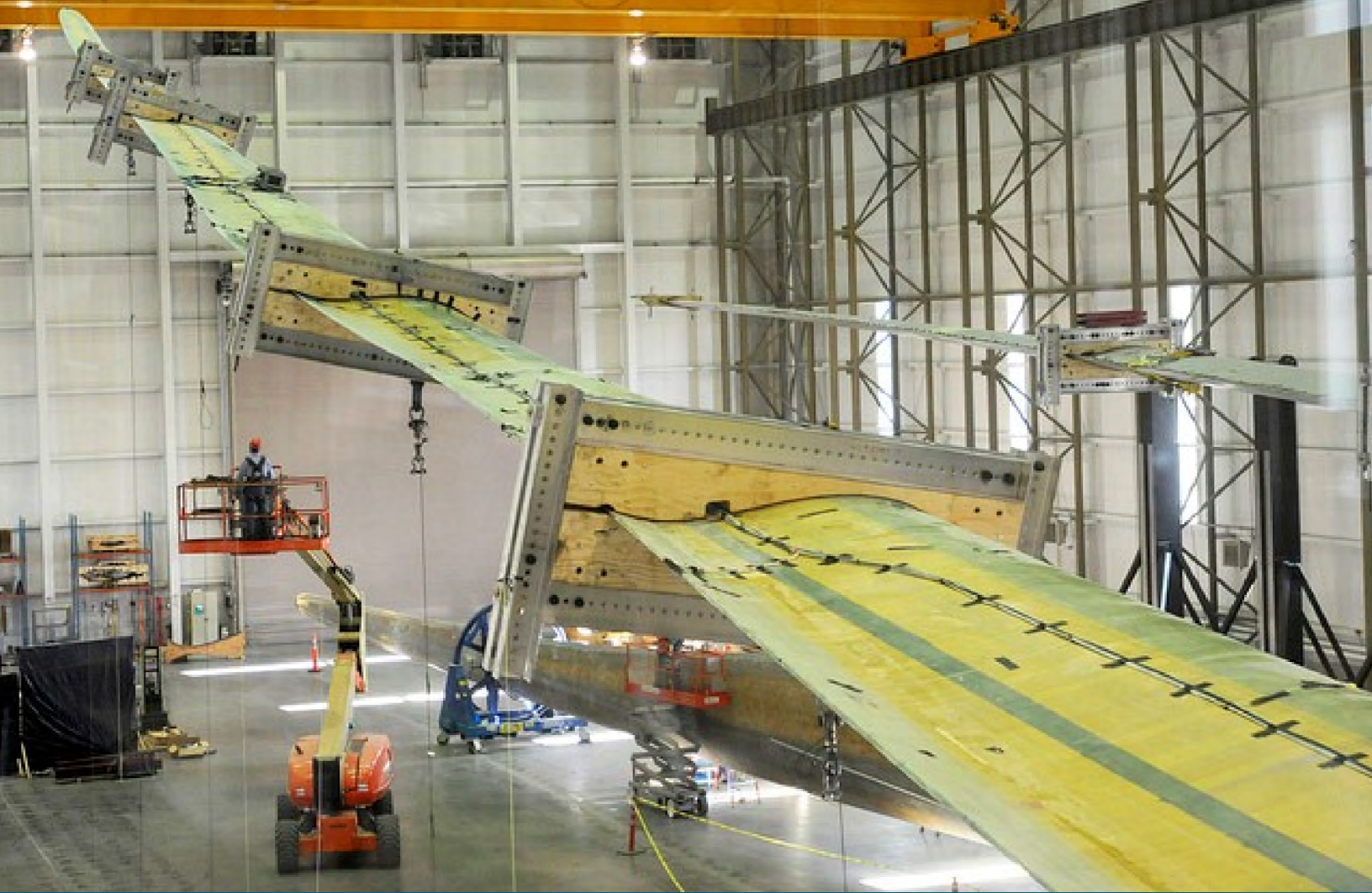
A prototype wind turbine blade is prepared for tests at Massachusetts Wind Technology Testing Center in Charlestown, MA. Photo: Massachusetts Clean Energy Center
