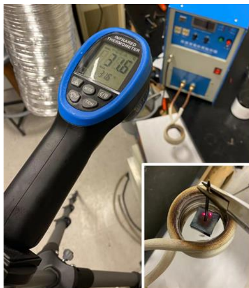
Figure 2. Temperature measurement setup for MIH. The inset shows the laser points of the thermometer on the iron sheets. A tripod is used to fix the thermometer during the measurements.
