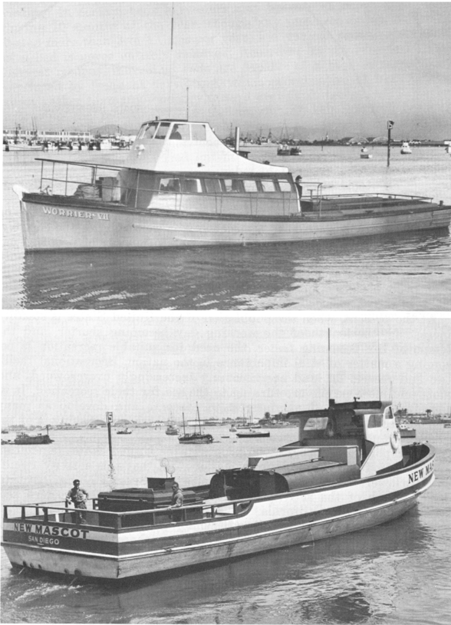
FIGURE 54. Examples of party sportfishing boats (partyboats). Top: Worrier VII carries 23 passengers, is 48 feet long, and is powered by 450 hp twin diesel engines. Bottom: New Mascot carries 60 passengers, is 65 feet long, and is powered by 600 hp twin diesel engines. Courtesy H & M Sportfishers.
