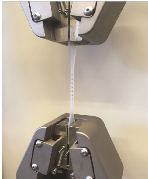
Figure 57: Uniaxial tensile testing of ethylene vinyl acetate tube material [MTS-Criterion tester]. The initial length of the specimen is l_0 = 140 mm, and the initial dimensions of the rectangular cross section are 3 mm x 1.59 mm.
